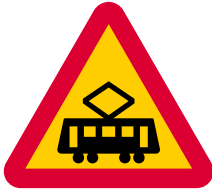
Junction with tramway line (A37)
