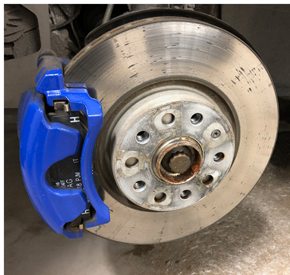
Wheel removed from a car with disc brakes. The brake caliper is the blue part.
