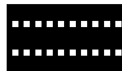
Road marking for bicycle passage (M16)
