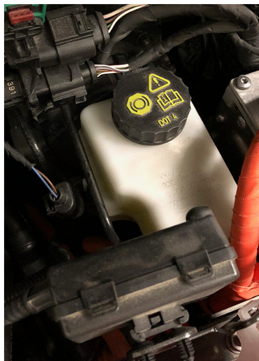
Brake fluid is normally yellow.
